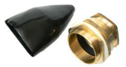
The Termination Technology range of BW 2 Part brass cable glands suitable for steel wire armour (SWA) cable. Suitable for indoor application, all packs supplied complete with glands, LSF shrouds, galv locknuts and brass earth tags. Smaller sizes up to and including BW32PK are supplied in packs of 2, BW40PK and above are supplied in packs of 1. CW gland packs are also available as well as LSF versions in both ranges
