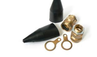
The Termination Technology range of CW Brass cable glands suitable for termination steel wire armour (SWA) cable. Suitable for outdoor application, all packs supplied complete with glands, PVC shrouds, galv locknuts and brass earth tags. Smaller sizes up to and including CW32PK are supplied in packs of 2, CW40PK and above are supplied in packs of 1. BW indoor gland packs also available as well as LSF versions of both ranges.
