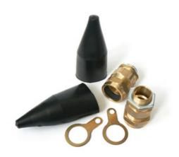
The Termination Technology range of CW Brass cable glands suitable for termination steel wire armour (SWA) cable. Suitable for outdoor application, all packs supplied complete with glands, PVC shrouds, galv locknuts and brass earth tags. Smaller sizes up to and including CW32PK are supplied in packs of 2, CW40PK and above are supplied in packs of 1. BW indoor gland packs also available as well as LSF versions of both ranges.
