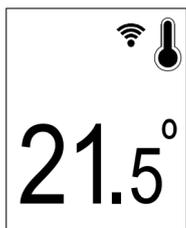
When in Easy mode the screen will change to show the current room temperature. The temperature required can be set with the **▼** and **▲** keys and switch the radiator on or off with the **Standby** key. None of the other keys or functions are available.
