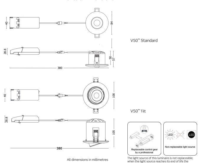
luminaire shall be replaced, utilising the existing driver.
