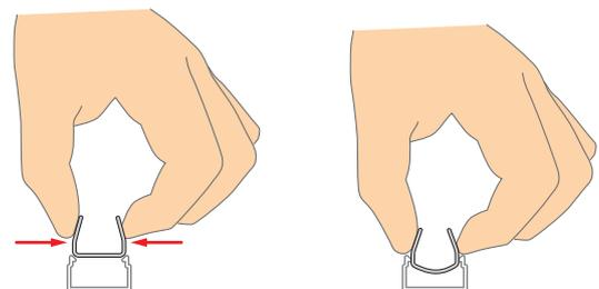
When inserting U-Clip 30 in 25x16mm trunkings, gently nipping the upright tabs causes the base to compress for tight fitment in the trunking.
