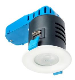
A low energy Fire Rated Downlight fitted with dimmable GU10 LED lamps, rated at IP65. Versions available with lamps in either 2800K or 4000K colour temperature options, and fittings have a choice of white, chrome or satin chrome bezels
