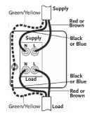
2. Any bare earth conductors must be sleeved with green/yellow sleeving.
