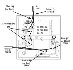
If earth conductors are bare, they must be sleeved with appropriate green/ yellow sleeving. If you are in any doubt about connecting this product consult a qualified electrician. Wiring insulation tests should be completed before setting the SafetySure RCD Spur to avoid misleading instrument readings and possible internal damage to the unit.
