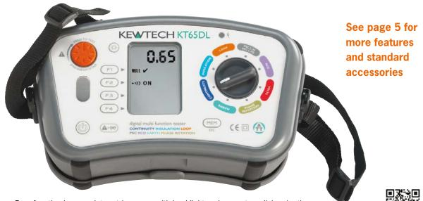
Four function keys, a dot matrix screen with backlight and one rotary dial make the KT65DL the easiest to use MFT
