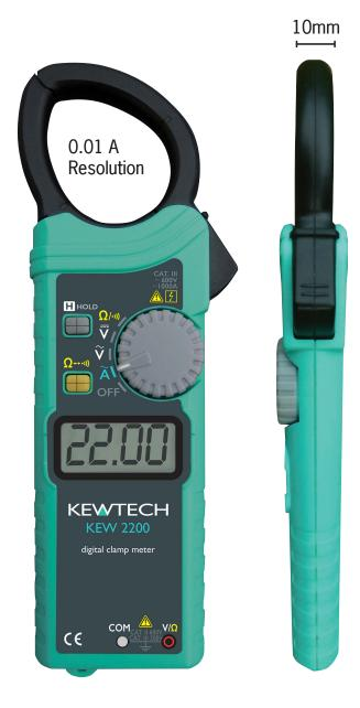
From the market leaders in Clamp Meters the KEW2200 represents another first. This 1000A clamp has jaws that are only 10mm thick and together with the tear drop shape makes for easy access into distribution boards and cramped spaces and also reads down to 0.01 A.
