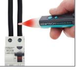
To distinguish between two cables close to each other press and hold down the attenuation switch, the Kewstick will be desensitised and has to be held closer to the cable to respond to the electrical field. This way you can differentiate between line and neutral or dead cables when they are close to each other.
