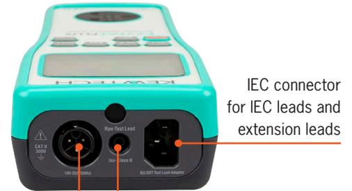
IEC connector for IEC leads and extension leads
