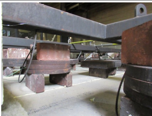
Photograph 16: Example of loading system.
