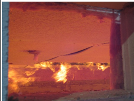
Photograph 29: During the test after 27 minutes – first piece of gypsum board falls into the oven.
