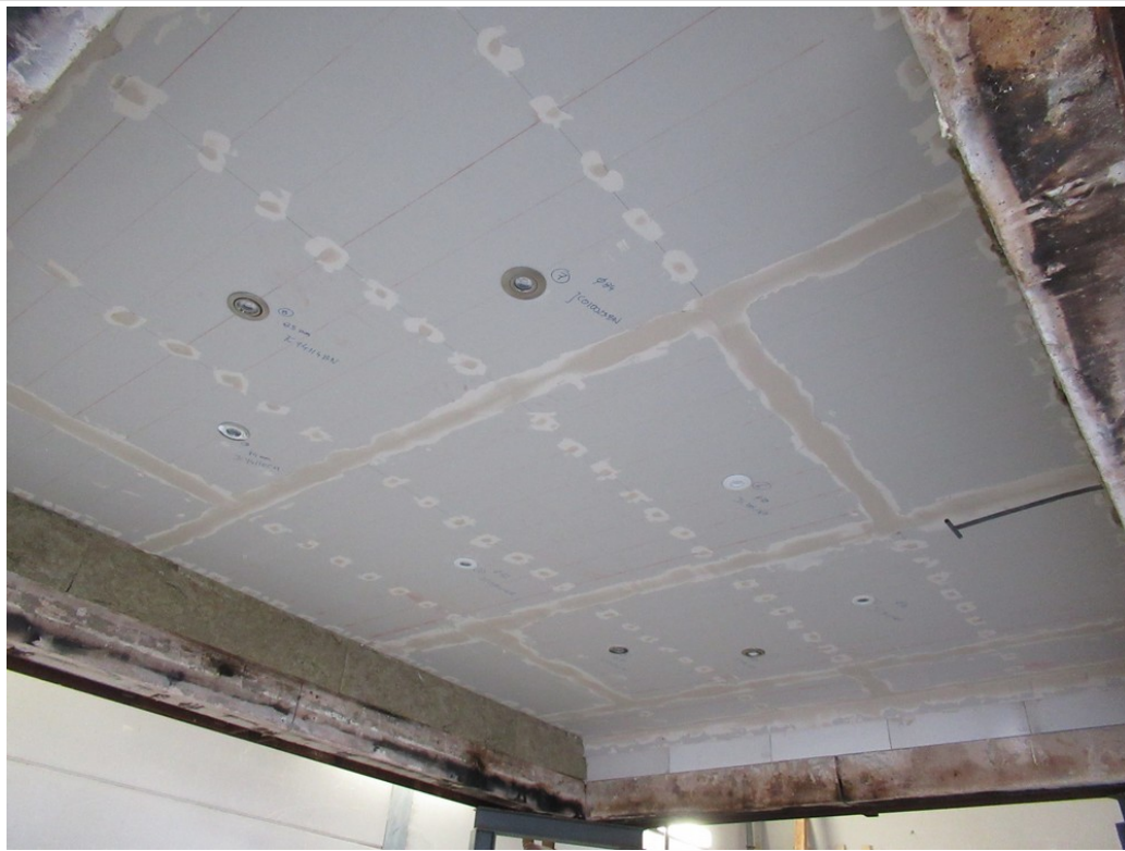
Photograph 15: Exposed side before the test with all six downlights installed in the ceiling.
