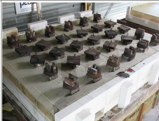
Photograph 17: Top view on the loading system.
