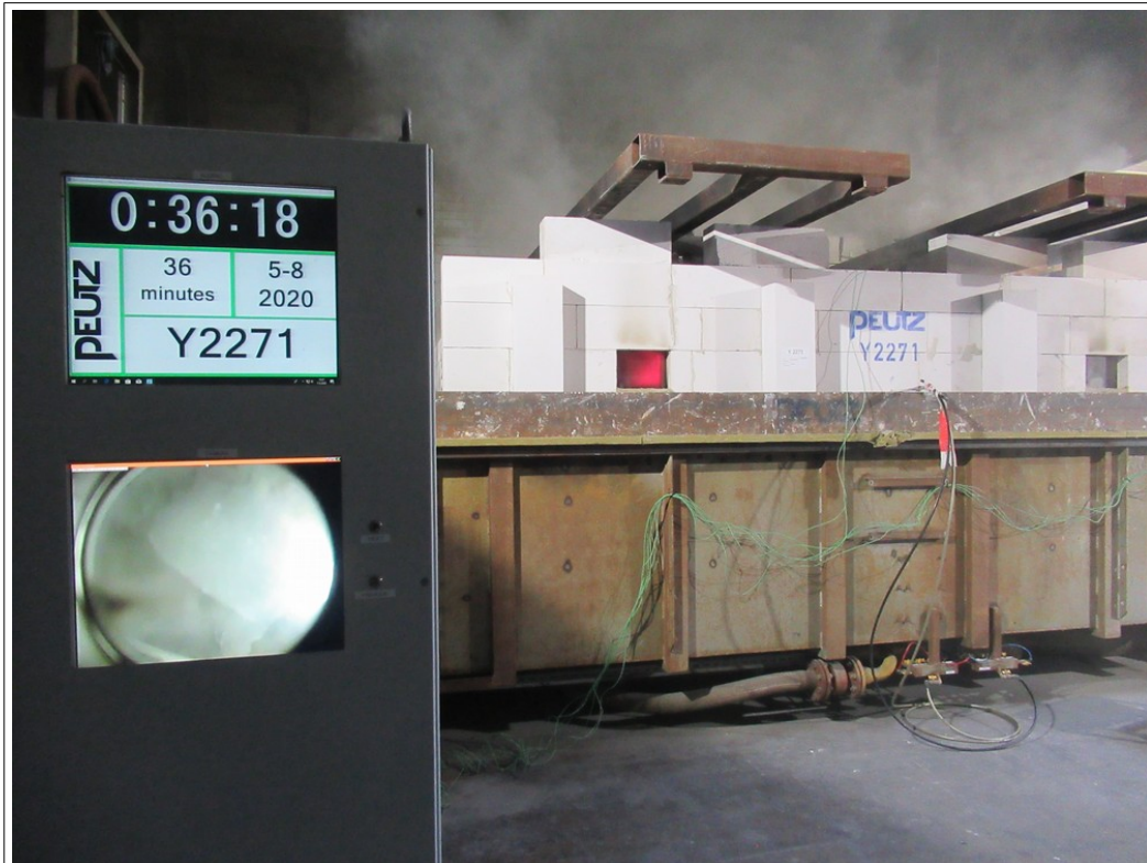
Photograph 33: During the test after 36 minutes: seconds before floor construction collapses.
