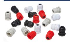
IP65 / IP68 rated (With neoprene washer sold separately (see page 35) Manufactured from nylon / Low smoke / Halogen free / Locking nut included / Dynamic state -20°C to +80°C, intermittent to +100°C
