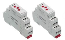
EN61812-1 / EN61010-1 IP40 for front panel / IP20 terminals Output: 2 x SPDT Current rating: AC-1 @16A. Modular width: 17.5mm. Din rail mounting. Operating temperature -20 +55°C
