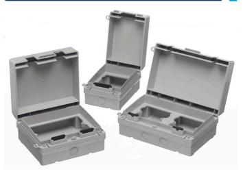
Accommodates standard socket, spur, switches and RCDs / 20mm cable entries located top, bottom, side and back / Grey enclosure / Corrosion resistant / Padlockable for added security (1 padlock). The ECWSK1 & SK2 have an improved design to accommodate most styles of 13A sockets and moulded plugs.
