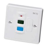
30mA trip / Test facility / ON/OFF indicator / Rated voltage 240V, 50Hz Rated current 13A / Trip time less than 40mS / Mechanically latching (Passive) / Spur will not trip in the event of a power failure
