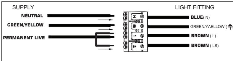
**Maintained (Switched) Wiring:** The product is used as a normal light - switch on/off, light turns on/off. Comes on during a power failure.
