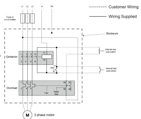
Additional start and stop stations can be wired to the DOL control circuit. In principle, the start buttons should be momentary normally open device and wired in parallel with terminals 17 & 18.
