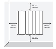
**WARNING:** The product is IP 24 rated and may be used in bathrooms, but not near baths, showers, water connections, basins etc. It can only be installed outside of zone 1 and 2. The product must not be installed where itself or the control panel is within the reach of persons in water.
