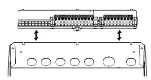
Pull and lift the terminal bar support away from the unit resting the rail supported by the earth strap. After fixing conduit/ cable glands, locate the rail support and press down.
