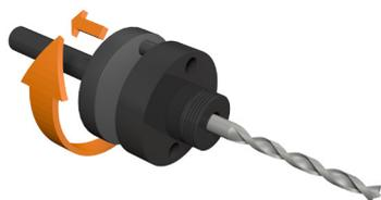
Take the adaptor and turn the knurled ring anti-clockwise to retract the drive pins into the position shown.
