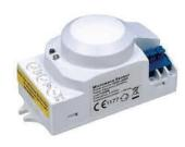
The Hispec microwave sensor is an active motion detector, it emits a high-frequency electro-magnetic wave (5.8 GHz) and receives their echo. The sensor detects the change in echo from even the slightest movement in its detection zone, which in turn triggers the 'switch light on' command.
