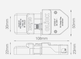
Dimensions: 105mm x 50mm x 23mm Cable Size: 4 x 1mm<sup>2</sup> Flex / 3 x 2.5mm<sup>2</sup> Solid Rating: 20A
