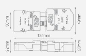
Dimensions: 135mm x 49mm x 23mm Cable Size: 4 x 1mm² Flex / 3 x 2.5mm² Solid Rating: 20A
