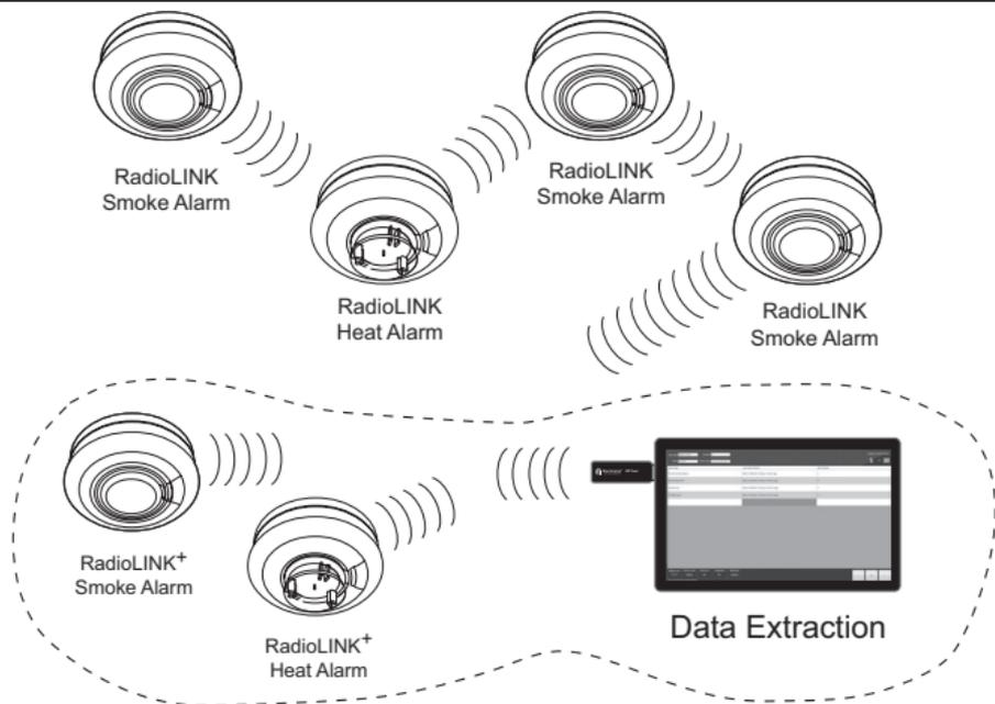
Note: Remote House Coding / Monitoring / Data Extraction only available on RadioLINK<sup>+</sup> Alarms
