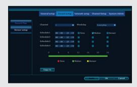
NB. When entering the 'Record Setup' the default screen will always start with a display of the settings for Channel 1 and the current day's schedule.
