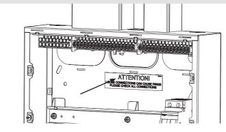
Rear cable entries shall enter thorough selected rear Knockout; once the Knockout is removed apply the appropriate cable entry plate (full list on page 4). Cable entry plates are available to clip into the knockout hole and provide a safe edge to bring cables in.
