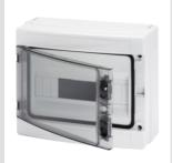
IP65 range of watertight anclosures from 4 to 72M with smoked transparent door. The main technical features are: reversible front and back panel, removable frames and panels with windows and detechable doors with up to 180° opening and lock accessory. The enclosures can be equipped with bipolar and unipolar terminal blocks, 80 A and 125 A, with screw wiring; they allow to create simple and neat wiring reducing the set-up time of the enclosure.
