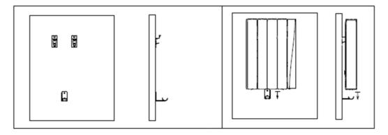
4. Secure the unit on the upper brackets by feeding the locking screws into the brackets as below.
