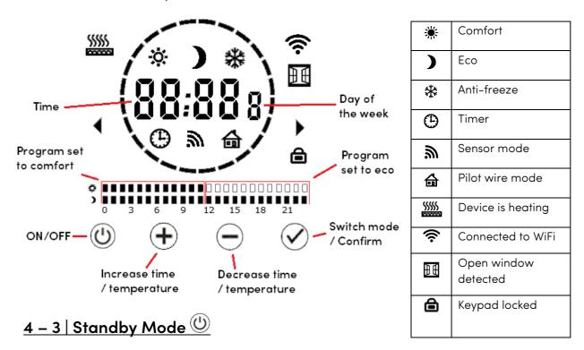
When the radiator first switches on it appears in standby mode, where the time is displayed and the radiator will not heat. You can use the button to switch between standby and the heating modes. When the radiator first turns on, the time will appear as 00:00. You can set the correct time in timer mode, see **4–4–4**.
