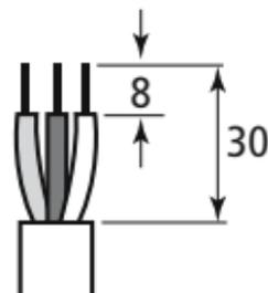
**Note:** When stripping the cables please use the measurements shown.
