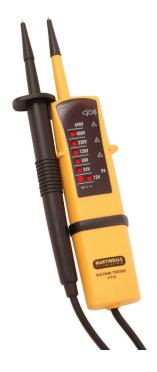
The VT12 is a two pole Voltage Indicator & Continuity tester with automatic AC/DC detection up to 690V and continuity testing with optical and acoustic indication up to 500k Ohms.
