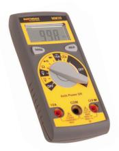
The MM39 is an auto-ranging multimeter with a large rotary switch for easy selection of the required test, even when wearing gloves. There are two test buttons, one to lock the range and the other to hold the results which are displayed on a 3½ digit LCD screen.
