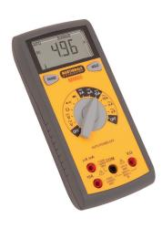
The MM65 is an autoranging digital multimeter which measures AC and DC voltages up to 600V, and AC and DC currents of up to 10A. It measures resistance to  $34 M\Omega$  and has a diode test and an audible continuity test which sounds below  $35 \Omega$ .
