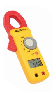
The CM55 is a new pocket sized high performance AC Clamp meter measuring AC current, AC/DC voltage and resistance with continuity test. The compact rugged design enables accurate and reliable current measurement down to 10mA resolution without the need to break into the circuit.
