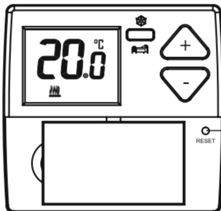
Press the Reset button located beneath the drop down flap
