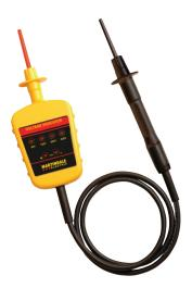
The VI-13800 provides instant visual AC and DC voltage indication in four stages from 50V to 400V. The bright long life LED indicators give clear and immediate display of the voltage level range. It has retractable probes, heavy duty finger guards and a two layer double insulated cable with a white inner core to give clear indication of damage that might compromise the user's safety.
