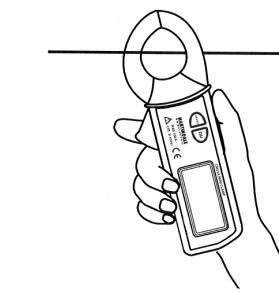
1. Press the POWER key to turn on the clamp meter.
