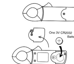
1. If the BAT symbol is displayed on the LCD then replace the battery.
