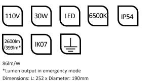
Dimensions: L: 252 x Diameter: 190mm Finish: Opal diffuser & yellow ABS body LED: 60/75pcs of SMD 2835 Working Temperature: -20°C - 40°C (0°C - 40°C for emergency version) H05VV-F 5m Cable included PG11 Cable Glands included Tripod available to order separately
