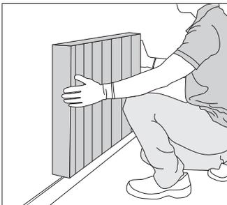
5. Slide product into fixed brackets, using a top to bottom method. Lift the product higher than the bracket and slide downwards into position.
