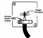
Each coaxial cable should be connected to the appropriate terminal as shown.
