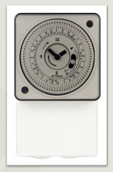
OP-IHTGPW IS A CAPTIVE-TAPPET 7 DAYIMMERSION HEATER TIME SWITCH. EACH TAPPET OPERATES FOR 2 HOURS. THE TIMER IS SUITABLE FOR SURFACE MOUNTING. THE 7 DAY DIAL CONTROLS A VOLT-FREE CHANGEOVER SWITCH, WITH A RESISTIVE RATING OF 16 AMPERES. PRE-FITTED (REMOVABLE) LINK FOR MAINS SWITCHING.
