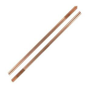
These copper bonded earth rods are made from low carbon steel of grade BS 970 or AISI 1018 with a high tensile strength of at least 600 N/mm2. The low carbon steel core is molecularly bonded with 99.9% pure electrolytic copper.
