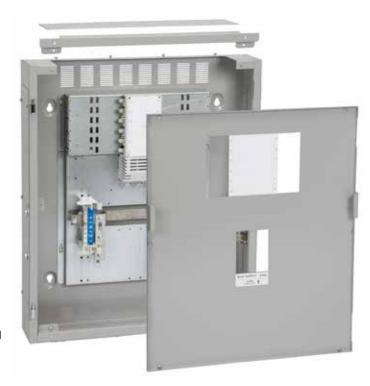
Option to remove top and bottom cross rails provides the ability to lay cables into the board instead of feeding them through the gland plate aperture, resulting in big time savings.
