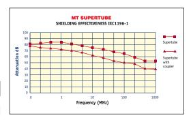
The graphs above show that the shielding effectiveness of MT Supertube is highly effective throughout the entire frequency range and will provide protection from interference for data, telecoms and signal cables.
