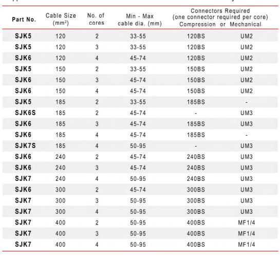
All joints are supplied with clear mould, resin pack, earth continuity, gloves, sealing tape.
