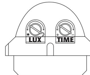
**ADJUSTING THE DURATION TIME:** the length of time that remains switched on after activation can be adjusted from (10±5) seconds to (4±1) minutes; rotating the TIME knob from (+) to (-) will reduce the duration time.
