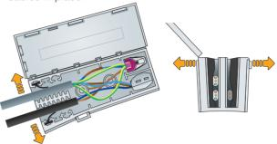
7 Try to keep cables of a similar size together in the same slot and simply push them into the slot as far as they will go.
