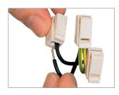
1. Strip both conductors 9 - 11mm. 2. Insert the solid conductor fully into the installation side.
