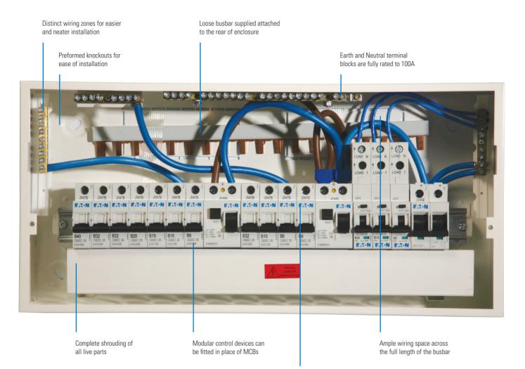
Freely configurable RCD ways on split load boards
