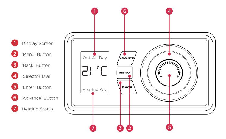
The heater is fitted with an adjustable thermostat enabling the room temperature to be controlled. The minimum room temperature is 7°C. The maximum temperature is set to 30°C by default. A temperature of 21°C is a common comfortable room temperature.
