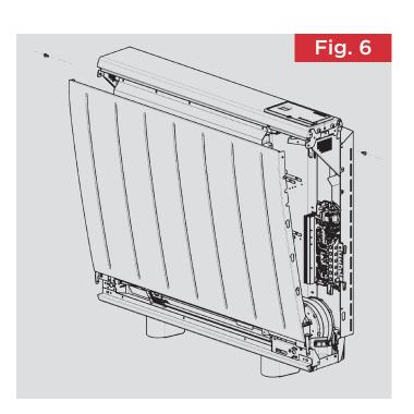
**6**. Remove the two screws securing the front panel, located at the upper sides of the heater, and swing the upper edge of the front panel upwards and unhook it from along the heater base.
