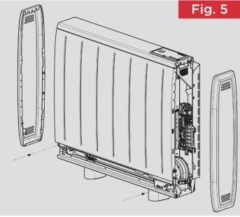
**5**. Remove the two screws located towards to bottom of either end of the heater, which retain the heater sides.
